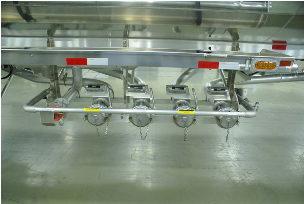
DOT 406 External loading lines.
