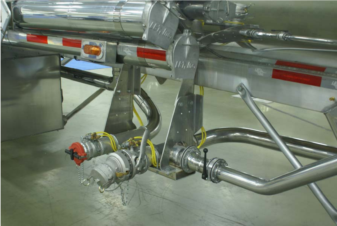
DOT406 trailer with just one compartment. Used for such things as crude oil and jet fuel.
