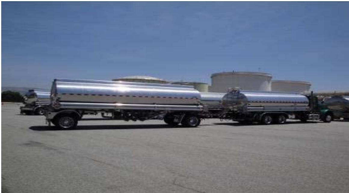
This is a typical truck and trailer combination which is commonly used on the West Coast. The external piping on the pull or pup trailer is more exposed than the piping on the truck mounted tank. It would appear that this unit would need a purging system on the pull trailer but not on the tank truck.
