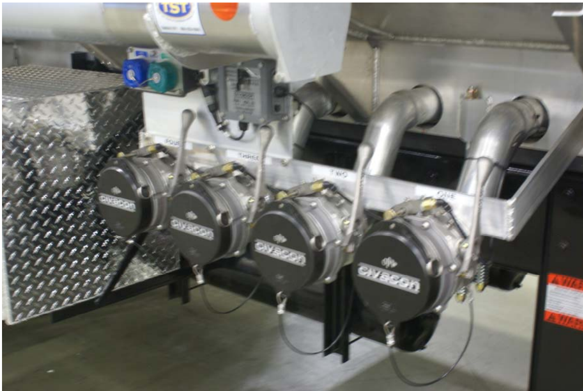
External loading lines on DOT406 straight truck.
