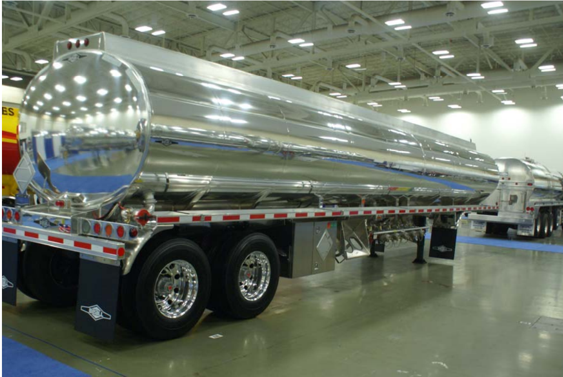
DOT 406 semi-trailer. Typically up to 9,000 gallon capacity with four to five compartments to allow transportation of different grades of gasoline or petroleum products.
