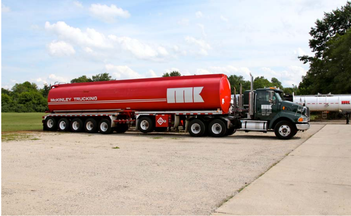
This is a Michigan style DOT406 trailer which can haul up to 12,000 gallons because of the extra axles. The axles provide a protective barrier to all but a direct impact on the external piping.
